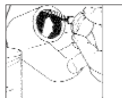
REF 107TA8514 Non hardening sealant which forms an elastic film
