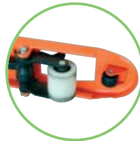
Single fork wheels: better for lightweight loads
