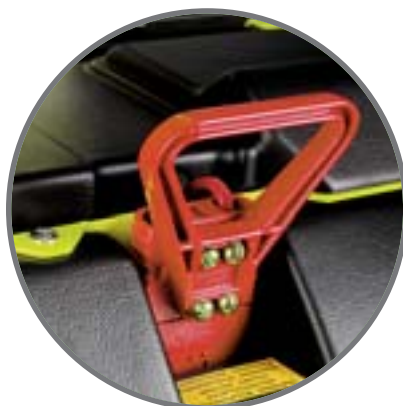
Solid central battery connector - easy to disconnect
