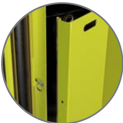
Side opening for easy battery replacement
