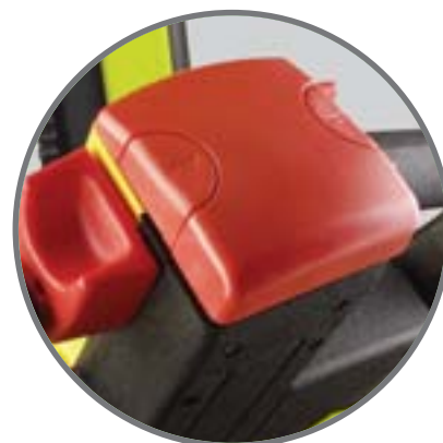
Emergency stop, horn and buttons for precise speed regulation
