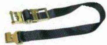
REF 124TA2791 Length : 1,15 m Capacity : 1500 Kg Assembly strength: 750 Kg With safety hook Not for lifting
